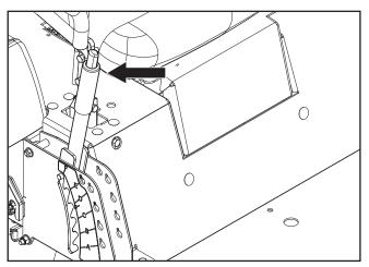
Mower deck lifting lever
